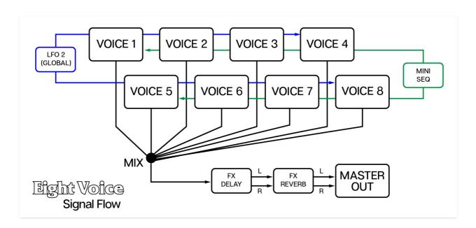
The voice modules themselves bear a great resemblance to the original Oberheim SEM modules of the 70s. Each of these features two oscillators, a state-variable filter with continuously variable lowpass-to-highpass response
