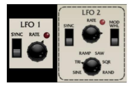
Eight Voice includes two low-frequency oscillator (LFO) that generates subaudio range signals intended for modulation purposes. Actually, Eight Voice has nine LFOs: one for each of the eight voice modules (LFO 1), and a global LFO for the entire instrument (LFO 2). We'll go over LFO 1 and LFO 2 separately as they differ a bit.
