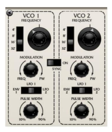
The voice modules each contain two almost identical voltage-controlled oscillators. The only difference are their modulation routing options.
