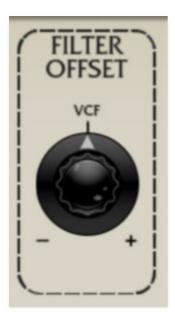
This acts a master filter cutoff control for all eight voices. Moving does not affect the actual knob positions - like the original instrument's offset knob, it adds or subtracts CV from the cutoff setting of all modules, with the center position being zero. We recommend assigning this to hardware knob or slider control, or the mod wheel (see the MIDI Controllers Setup and The MIDI Tab section for information on how to do this; it's really easy).
